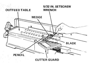
5. If a cutter blade adjustment is not required, check each locking screw of each wedge (5/32" setscrew wrench) and tighten if necessary. Hold the pulley while tightening screws and be careful that your fingers do not slip off the wrench."
